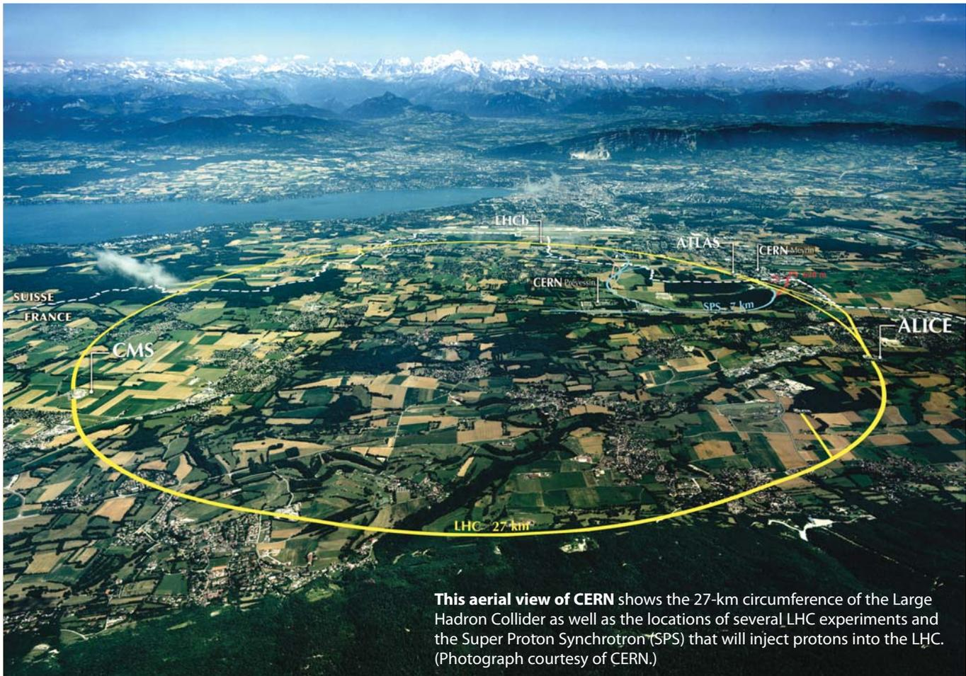
This aerial view of CERN shows the 27-km circumference of the Large Hadron Collider as well as the locations of several LHC experiments and the Super Proton Synchrotron (SPS) that will inject protons into the LHC. (Photograph courtesy of CERN.)
